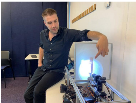
Emanuel Larsson illustrates how the latest version of his kitchen-based light tomography (KBLT) scanner works. Photo: Noomi Egan.
